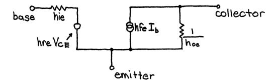
Utilizing the h-parameters, the h-parameter common emitter equivalent circuit, ohms and watts law, and the formula for parallel resistors, we shall solve for Ai, Av, Zin and Zout.
