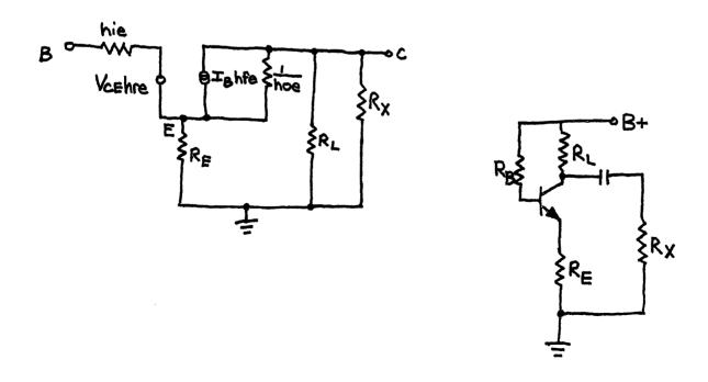
Current gain is equal to the change in output current  $(I_{out})$  divided by the change in input current  $(I_{IN})$  which gives us:
